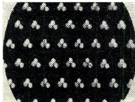
Fig. 9. Dot pattern when the d.c. convergence voltage is too high. Here, the blue dot is on top with the red to the left and the green to the right below.
